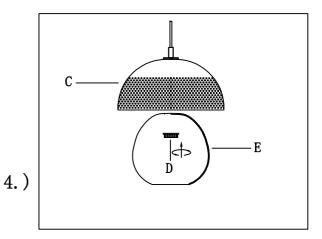
Step. 4: Use socket ring (D) to secure glass shade (E) on body.
